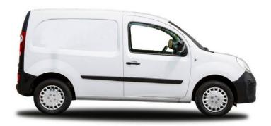
**N1:** Vehicles designed and constructed for the carriage of goods and having a maximum mass not exceeding 3,500 kg. e.g., light vans and trucks. **CVRT** tested annually.
