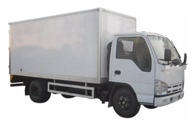
**N2:** Vehicles designed and constructed for the carriage of goods and having a maximum mass exceeding 3,500 kg and not exceeding 12,000 kg e.g., larger vans and trucks. **CVRT** tested annually.
