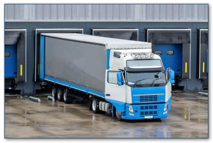
**N3:** Vehicles designed and constructed for the carriage of goods and having a maximum mass exceeding 12,000 kg e.g., trucks. **CVRT** tested annually.
