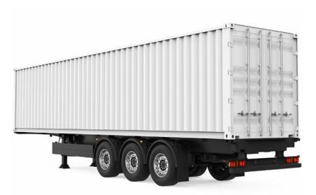
**03:** Trailers with a maximum mass exceeding 3,500 kg but not exceeding 10,000 kg. **CVRT** tested annually.
