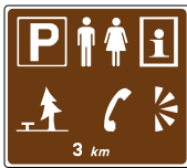
Advance sign for facilities in lay-by
