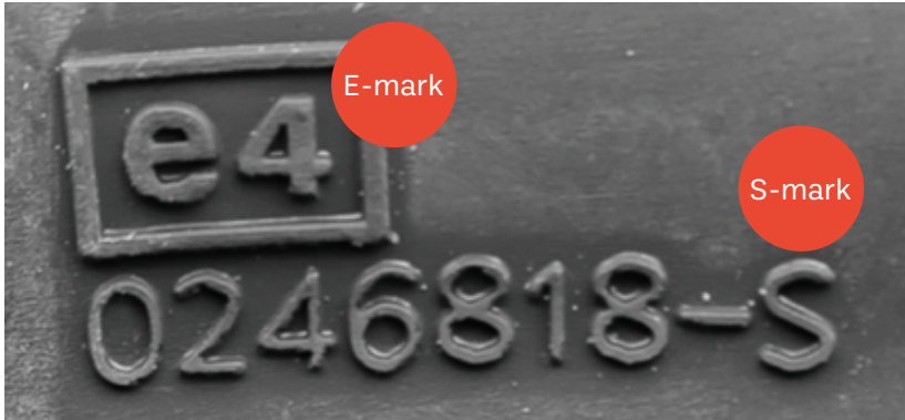
Figure 2: E-Mark and S-Mark on tyre sidewall
