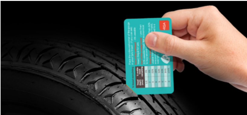
Figure 5: How to use the handy pop-out tyre tread depth gauge.
