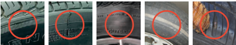
Sidewall Tear Sidewall Cut Bulge Exposed Plies Penetration Damage
