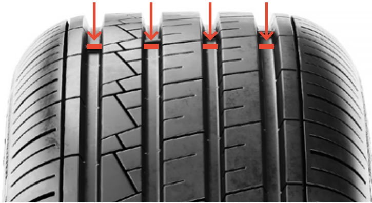
Figure 3: Tyre wear indicator
