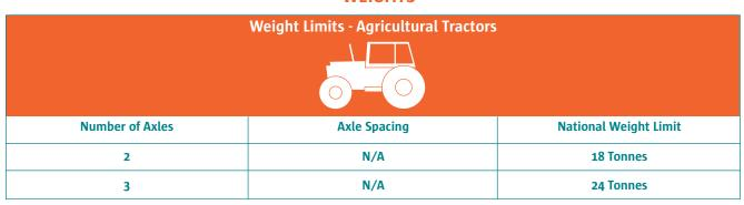
Note: Combinations of agricultural tractors and trailers, where either of them is unplated are not allowed to tow more than three times the tractors unladen weight.
