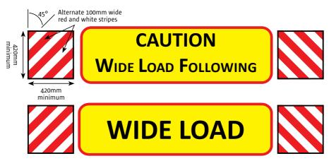
Figure 20: Wide Load Signage to be used when transporting self-propelled equipment over 3.5 metres wide on public roads.
