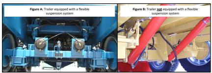
Figure 16: Images of a trailers equipped with or without flexible suspension systems.
