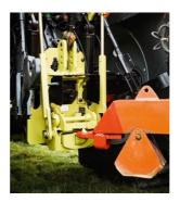
Figure 12: Image of 'hook and ring' type coupling. (Image courtesy of Dromone Engineering)
