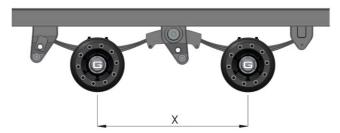
Figure 2: Axle Spacing (Image Courtesy of Granning Axles)
