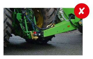
Figure 18: Incorrectly fitted safety chain. (Image courtesy of Dromone Engineering)
