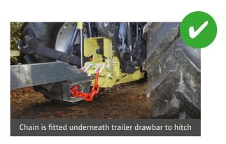
Figure 17: Correctly Fitted Safety Chain. (Image courtesy of Dromone Engineering)
