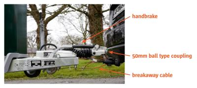
*Figure 1: Image of 50 mm ball-type coupling.*
