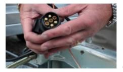
Figure 17: pin lighting connector
