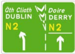
Lane destination sign
