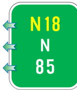
Example of dual carriageway LRI sign
