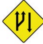
Start of a climbing lane
