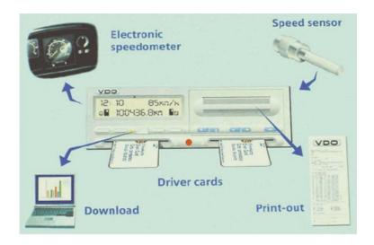
The motion or speed sensor is located on the gearbox. It signals in an encrypted form the vehicle speed and distance travelled by the vehicle for the VU to record. The VU and the motion sensor are paired and the signals from the sensor are fully encrypted. This means any attempt to interfere with them is detected and recorded by the vehicle unit.
